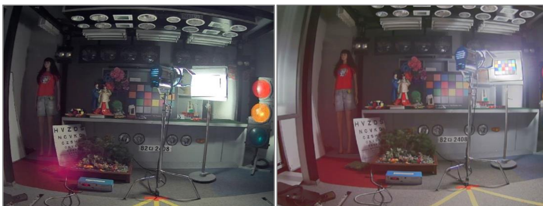
Image 2. Conventional WDR (left) and Wisenet5 WDR (right) comparison
