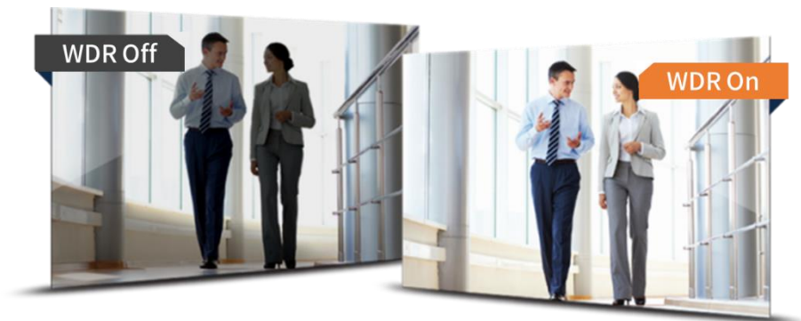
Image 1. WDR is applied when the main object is dark due to the bright background.
